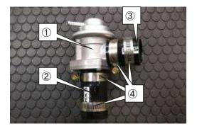
(6) Temporarily install ①Blow-off Valve assembled in (5) to ②Suction Pipe No.1.
