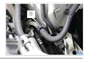
(10) Remove ①A/C pipe' clamp shown in the diagram.
