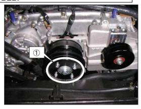
(2) Install the supercharger pulley using the provided Hexagon Cap Bolt. The supercharger pulley must be purchased separately and selected according to the target engine output.
