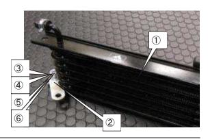
(3) Cut off the runover "A" from the Oil Cooler Bracket No.1 along the bracket.
