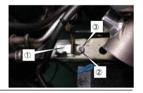
(3) Temporarily install the I/C Inlet Pipe No.1 to the installation position, and cut the portion "A" in the diagram that may come in contact with the pipe.
