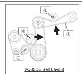
(5) <u>Tighten the four M6 bolts which were temporarily installed on @idler pulley No.2.</u>
