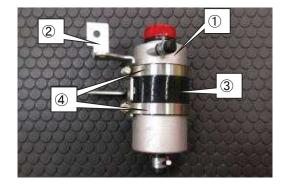
(9) Install ②canister purge control valve to ①Traction Oil Tank using a factory nut.
