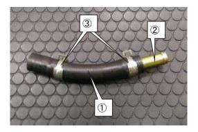
(7) Install ①Suction Hose to the factory blow-by hose (A) using a factory clamp and ②Hose Clamp 16mm.
