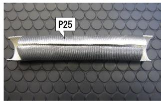
(6) Cover the hose with the Thermal Tube modified in (5). Secure the covered hose with a wire.
