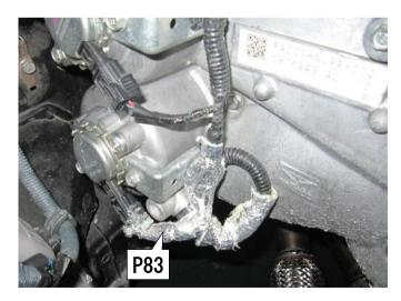
(3) Install the provided Insulator  $\phi$ 60 to the Extension as shown in the photo one the right, and secure it with the provided Hose Band #40.
