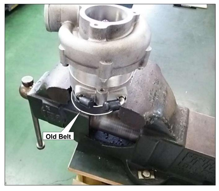
(2) Loosen the center bolt of the 1-hole S/C Pulley.
