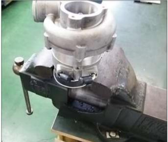
(8) Tighten the center bolt of the pulley.
