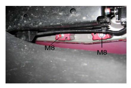
3. Remove 3 x M8 bolts from the canister mounting bracket. Note: Do not remove the canister because the solenoid harness is secured to the canister mounting bracket.
