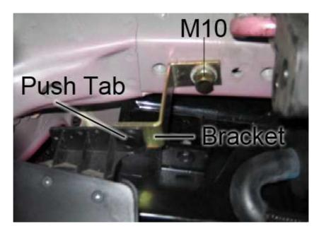
9. Install the bumper skin bracket (using the existing hole) with the supplied M10 bolt/lock washer/plate washer to the bumper skin reusing the stock push tab.
