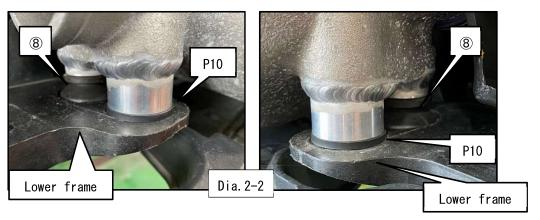
(2) Attach the intercooler bracket removed in 1. (4) to the lower frame.
