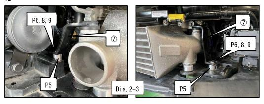
(3) Attach the inlet pipe to the intercooler core. (Dia. 2-4)
