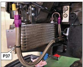
(27) Securely install the Oil Cooler Hose 1 to the Oil Cooler Core.
