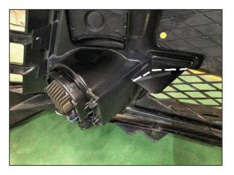
(18) Secure the wires shown in the diagrams below using the provided Tie Wrap S.
