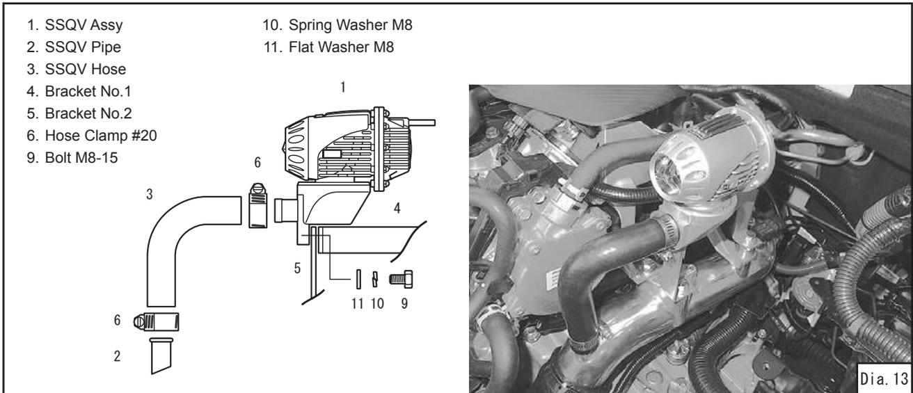
(9) Position the SSQV Assy where it does not come into contact with any other components.
