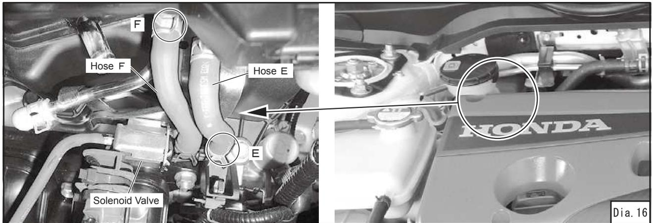
(16) Install the 6mm joint pipe and 6mm hose to the hose F. (Dia. 17, 18)
