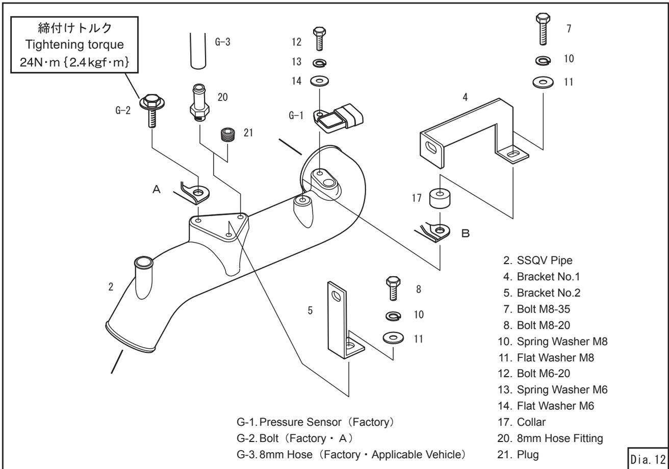
(8) Temporarily install the SSQV Assy. (Dia. 12, 13)
