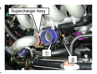
(32) Install the Elbow ① and Hose Fitting 10mm ② to Suction Pipe No.2; then, install the Silicone Hose 60mm L=70 ③ and Hose Clamp #36 to the pipe.
