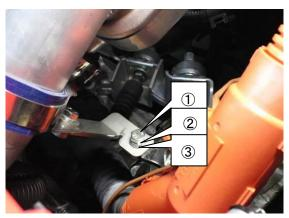
(21) Secure the Hose 8mm to ① using a tie wrap so the hose does not come in contact with other parts of the vehicle as shown the diagram on the right.
