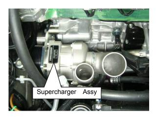
(12) Secure the Hose 8mm and 10mm to ① to ③ using tie wraps so the hoses do not come in contact with other parts of the vehicle.
