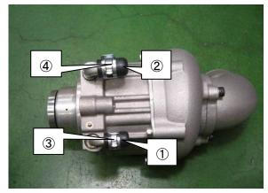
(10) Connect the 1000mm Hose 8mm ① and the 570mm Hose 10mm ② to the Supercharger Assembly using the 8mm Hose Clip ③ and the 10mm Hose Clip 10mm ④ removed from the Supercharger Assembly in (9).
