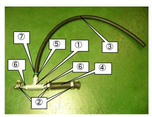
(24) Remove the factory vacuum hose, and install the 3 way fitting Assy between the intake manifold and factory vacuum hose.
