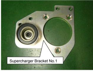
(5) Insert the Spacer M8 L=3.5 ② between the Supercharger Assy and the Supercharger Bracket. Install the Supercharger Assy to Supercharger Bracket No.1 using the Flat Head Bolt M8 L=35 ①.
