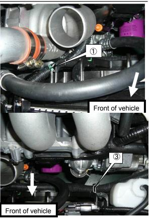
(13) Reinstall the factory intake manifold; then install Supercharger Bracket No.2 to the intake manifold using the factory bolt and Supercharger bracket No.1 with the following parts.
