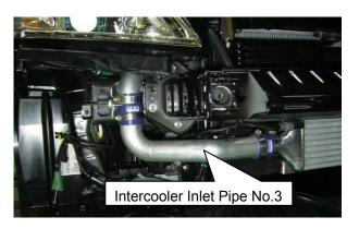
(11) Temporarily install Intercooler Inlet Pipe No.1 to the vehicle using the Silicone Hose 45mm-50mm ① and Hose Clamps #28 ②. After properly adjusting the positions of Intercooler Inlet Pipe No.1, 2 and 3, tighten all bolts and hose clamps temporarily installed.
