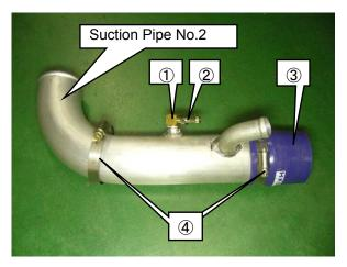
(33) Install the Restrictor ① to Suction Pipe No.2.
