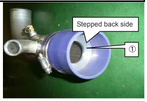
(34) Temporarily install Suction Pipe No.2 to the vehicle connecting the Hose Clamp #36 installed in (31).
