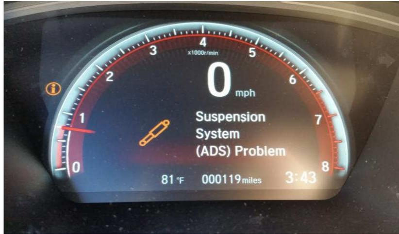
Once the stock suspension is removed, the control unit detects it as an error, and an error message appears as shown above.
