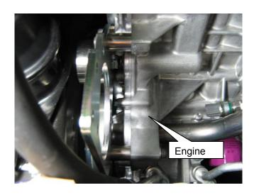
(3) Remove the factory engine oil level gauge. Cut the gauge as shown in the diagram on the right. Drill a hole on a tip and install the provided tie wrap to the hole to make a handle.
