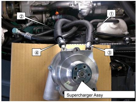
(8) Install the Supercharger Assy to Supercharger Bracket No.1 using ① Flat Head Bolt M8 L=35.
