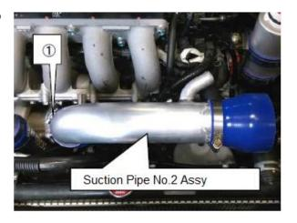
(35) Insert ①Spacer M4 L=1.5 between the airflow sensor removed from the factory air cleaner and Suction Adapter. Install the airflow sensor to the Suction Adapter using ②Button Bolt M4 L=12.
