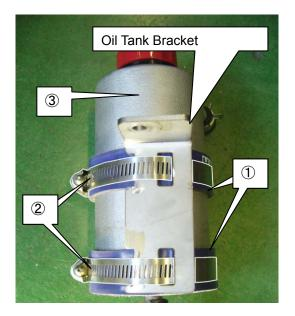
(6) Remove the rubber cap from the hose fitting on the lower part of the Oil Tank and connect the Hose 10mm ② using the Hose Clip 10mm ①.
