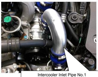
To Intercooler Inlet Pipe No.2
