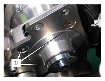
(9) Install the Supercharger Pulley to Supercharger Assy using ①Cap Bolt M6 L=12.
