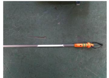
(4) Reinstall the modified factory engine oil level gauge back to the vehicle.
