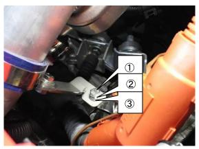
(20) Secure the Hose 8mm to ① using a tie wrap so the hose does not come in contact with other parts of the vehicle as shown the diagram on the right.
