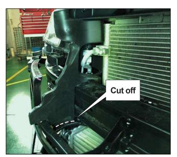
(15) Cut off the intercooler air guide LH along the dotted line shown in the diagram on the right.
