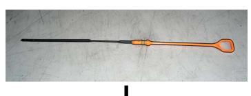
(4) Reinstall the modified factory engine oil level gauge back to the vehicle.
