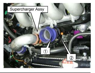
(31) Install ① Elbow and ② Hose Fitting 10mm to Suction Pipe No.2.
