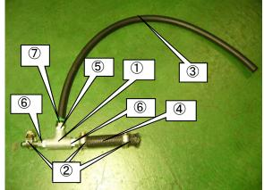
(23) Remove the factory vacuum hose, and install the 3 way fitting Assy between the intake manifold and factory vacuum hose.
