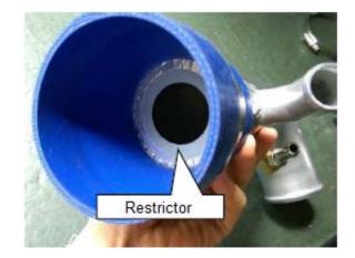
(34) Temporarily install the Suction Pipe No.2 Assy to the vehicle using the Hose Clamp #38 used in (33).
