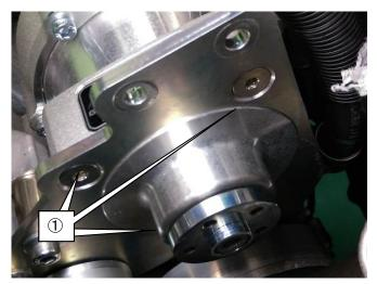
(9) Install the Supercharger Pulley to Supercharger Assy using ①Cap Bolt M6 L=18.
