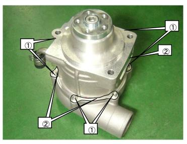
(6) Rotate the Supercharger unit and ③compressor Housing, and adjust the angle of the Supercharger Assy and compressor housing until there is 12mm gap between ④ the center line of the Supercharger Assy plate's both ends and ⑤ the center line of the compressor housing fixing bolt as shown in the diagram below. Retighten ①compressor housing fixing bolt and ②compressor housing fixing plate.
