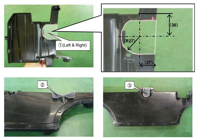
(27) Install the modified resin part of the factory front bumper air guide to the vehicle using the factory bolts and clips.
