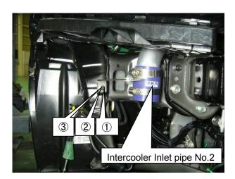
(10) Temporarily install Intercooler Inlet Pipe No. 3 to the vehicle.
