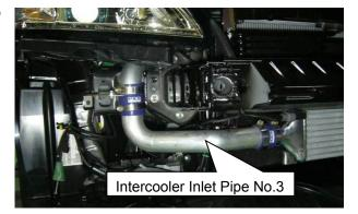
(11) Temporarily install Intercooler Inlet Pipe No.1 to the vehicle using ①Silicone Hose 50mm L=55 and ②Hose Clamps #28. After properly adjusting the positions of Intercooler Inlet Pipe No.1, 2 and 3, tighten all bolts and hose clamps temporarily installed.
