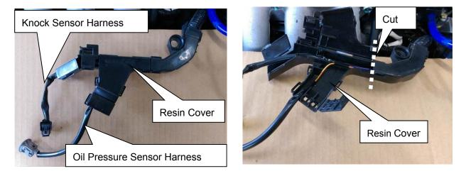
(13) After cut off the resin-made cover, cover the knock sensor harness and oil pressure sensor harness with the provided ① Corrugated Tube for Sensor Wiring. Secure the harnesses using the factory bolt as shown in the diagram below.
