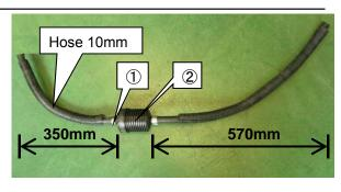
(5) Install the Oil Tank Bracket to the Oil Tank ③ using the Silicone Hose 70mm L=20 ① and Hose Clamp #40 ②.
