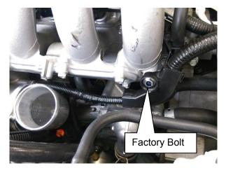
(14) Secure the Traction Oil Hose 8mm and 10mm with Tie Wraps at ①-③ in the diagrams on the right and below so the hoses do not come in contact with any other parts of the vehicle.
