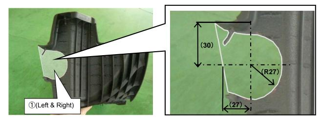
(29) Install the rubber part of the factory front bumper air guide to the vehicle.
