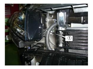
(15) Connect the 1250mm Hose 8mm 1 to the Oil Tank using the 8mm Hose Clip 2.
