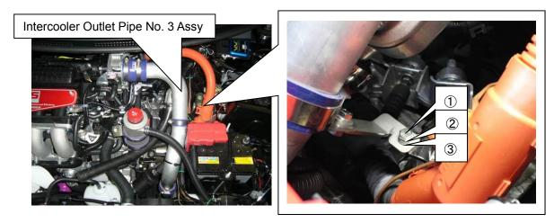
(20) Secure the Hose 8mm to ① using a tie wrap so the hose does not come in contact with other parts of the vehicle as shown the diagram on the right.
