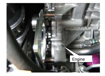
(3) Remove the factory engine oil level gauge. Cut the gauge as shown in the diagram on the right.Drill a hole on a tip and install the provided tie wrap to the hole to make a handle.
