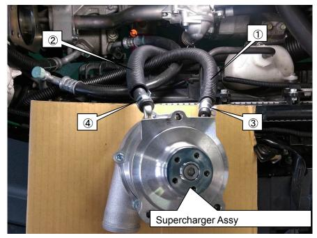
(8) Install the Supercharger Assy to Supercharger Bracket No.1 using 1 Flat Head Bolt M8 L=35.
