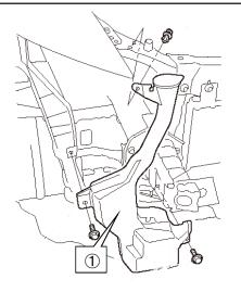
(18) Turn the auto tensioner pulley counterclockwise, and remove the belt. When turning the auto tensioner, use a tool ① such as Honda factory tool or box spanner. Place the tool as shown in the diagram on the right.
