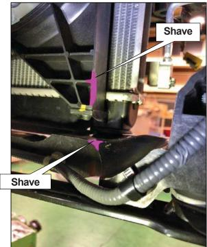
(14) Cut off the intercooler air guide RH along the dotted line shown in the diagram on the right.
