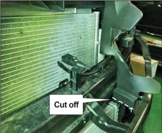
(15) Cut off the intercooler air guide LH along the dotted line shown in the diagram on the right.
