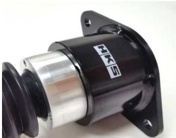
● The rear side is equipped with HKS original upper and high-strength billet aluminum bracket. Because of the way the force travels through the upper mount is different from stock suspension; other products that utilize stock upper mount are prone to develop noises overtime and malfunction. HKS uses a specially designed billet aluminum upper mount to ensure product quality and customer safety.
