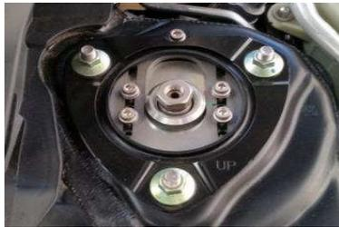
● Camber adjustable pillow upper is installed to the front side. The camber can be adjusted according to the tire size and/or driving conditions.
