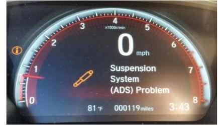
● The error message comes on when the stock suspension is removed. It can be canceled by installing an error canceller.
