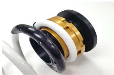
● The adjuster for the rear ID 65mm barrel spring allows the spring rate change which is usually impossible with the specially-developed spring. In addition to the original upper, the damping adjustment cable is included. Locating a dial of the cable to the inside of the wheel housings allows the damping force adjustment without lifting a vehicle that is usually required.
