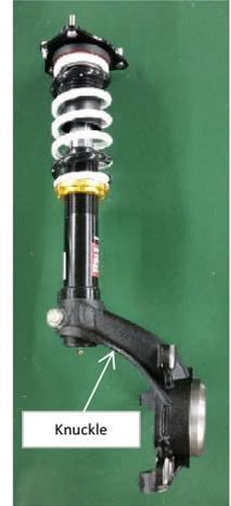
● **Rear: Single Tube Shock Body Length Adjustable Type**
