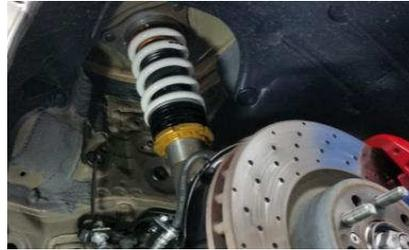
● High rigidity single tube inverted type is utilized for the front side to support sufficiently its weight and large bending load that is caused during acceleration, deceleration, and/or turning. It delivers outstanding durability that was achieved through our continued
