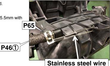
(6) Install the Hose Φ10② to nipple on cylinder brock.
