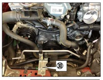
(35) Remove ③ Intake manifold. (Keep it for later use.)
