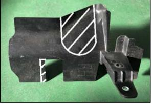
(24) Drill the  $\Phi$ 9mm hole(x2) to the Front bumper reinforcement.
