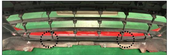
(15) Cut the 16 Intake manifold cover.
