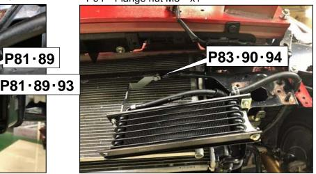
(19) Install the Hose  $\Phi 8$  (1) and (2) to the Supercharger & Traction fluid tank, and fix the hose  $\Phi 8$  (1) and (2).
