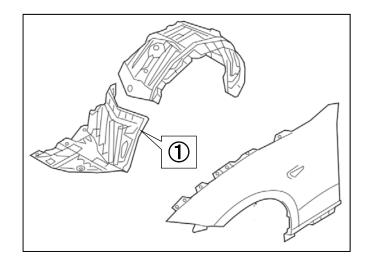
(5) Remove the 2Engine under cover 1.
