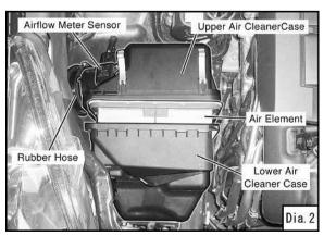
5) Loosen the bolt and nut; then, remove the lower air cleaner case. (Dia.3)
