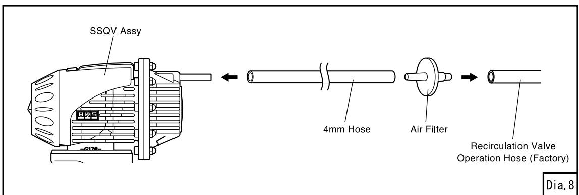
**The SSQV must be activated by intake manifold pressure.**
